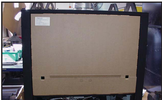
Figure 13.10 Splatter Guard with Lower Access Panel Open
